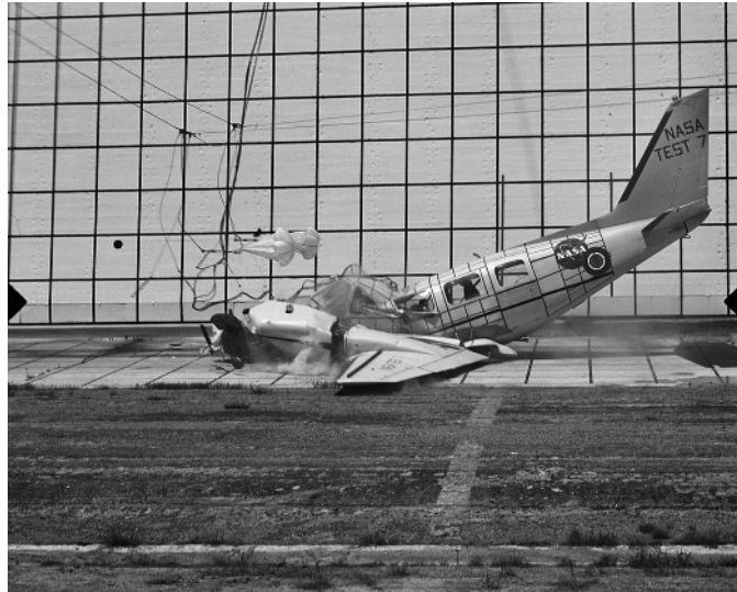
Figure 1.7 The Impact Dynamics Research Facility is used by NASA to conduct crash testing of full-scale aircraft under controlled conditions. The aircraft are swung by cables from an A-frame structure that is approximately 400 ft long and 230 ft high. (Source: NASA; http://commons.wikimedia.org/wiki/File:Impact_Landing_Dynamics_Facility_Crash_Test_-_GPN-2000-001907.jpg )
