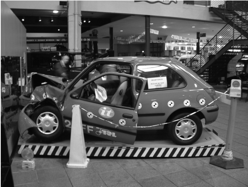
Figure 1.8 A crash test is a form of destructive testing usually performed in order to ensure safe design standards in crash worthiness and crash compatibility for various modes of transportation or related systems and components. There are various types of crash test, such as frontal-impact test (in the photograph), offset crash test, side-impact crash test, and roll-over crash test. (Source: StaraBlazkova at the Czech language Wikipedia [GFDL ( www.gnu.org/copyleft/fdl.html ) or CC-BY-SA-3.0 ( http://creativecommons.org/licenses/by-sa/3.0/ )], from Wikimedia Commons; http://commons.wikimedia.org/wiki/File:Muzeum_of_trans_Gla_crash_test.jpg )
