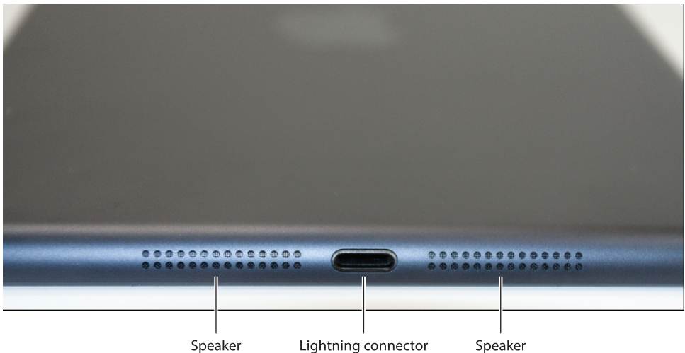
1.6 The bottom panel on the iPad mini houses two speakers and the Lightning connector.
