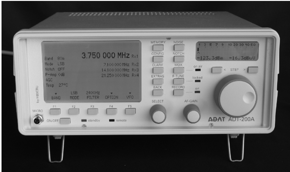
Figure I.21 ADT-200A is a first prototype of an almost fully digitized radio receiver (Digital RX of generation 2.5), designed as a stand-alone unit. Using a 14 bit A/D converter with a signal-to-noise ratio of 74 dB above half the Nyquist bandwidth of 36.86 MHz, in combination with the subsequent decimation it achieves a dynamic range (Section III.9.7) obtained so far only in high-end multiple-conversion superhets. A high-performance signal processor of the latest generation from Analog Devices having a processing power of up to 2 billion instructions per second performs the actual signal processing. (Company photograph of Hans Zahnd engineering consultants.)
