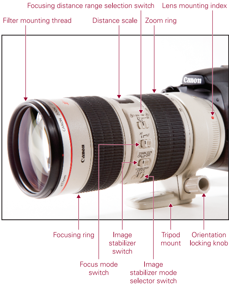
1.9 Lens controls, as shown on an EF 70-200mm f/2.8L IS USM.
