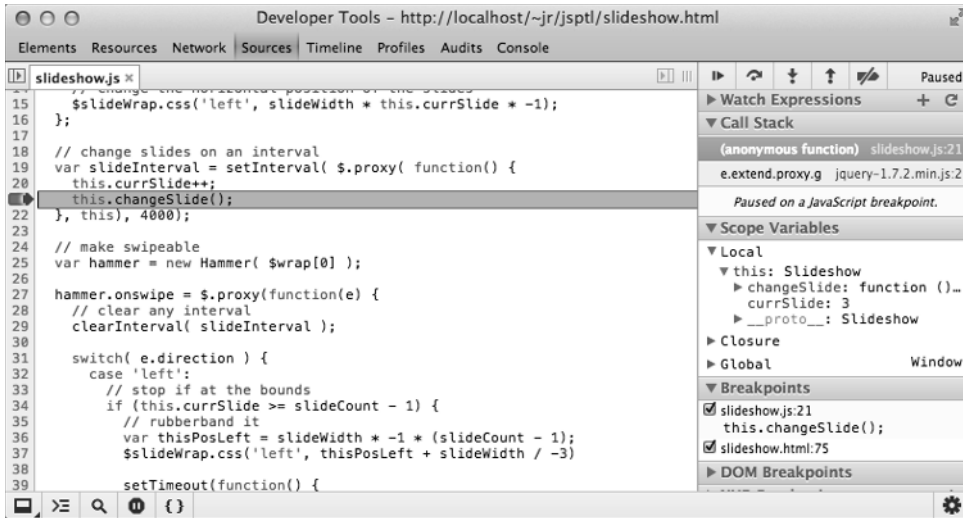
Figure 1-5 When the script reaches the breakpoint, you will be able to analyze the current value of any object.
