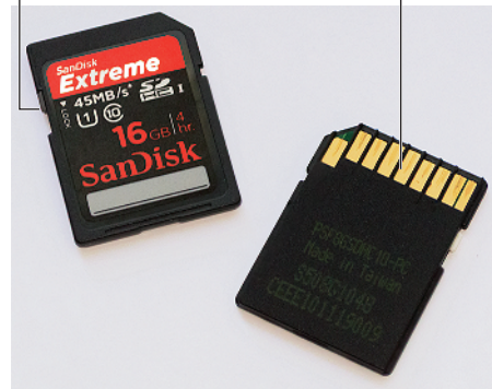
Figure 1-10: Avoid touching the gold contacts on the card.
