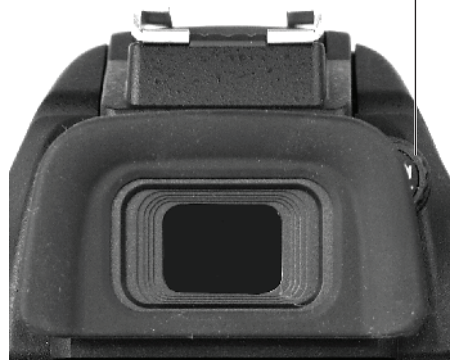
Figure 1-6: Use the diopter adjustment control to set the viewfinder focus for your eyesight.
