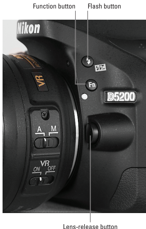
Figure 1-13: Press the Flash button to pop up the built-in flash when you shoot in the P, S, A, or M modes.
