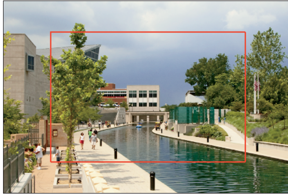
Figure 1-2: The 1.5 crop factor produces the angle of view indicated by the red outline.
