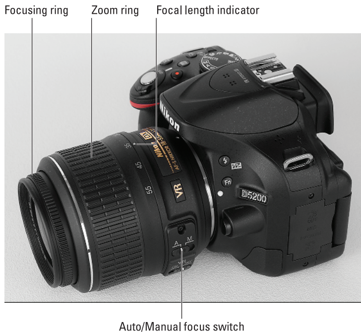
Figure 1-4: Set the focusing method (auto or manual) via the A/M switch.
