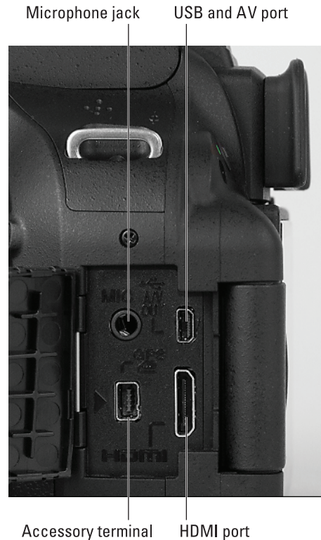
Figure 1-14: Open the cover on the side of the camera to reveal these connections.
