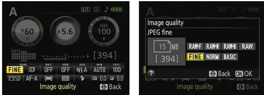
Figure 1-20: Press the Info Edit button to activate the control strip (left); highlight the option you want to adjust and press OK to display the available settings (right).
