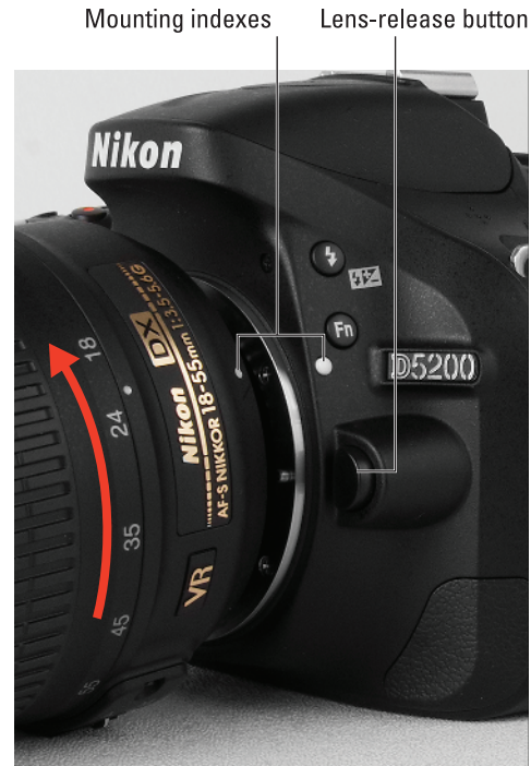
Figure 1-3: When attaching the lens, rotate it in the direction indicated by the arrow.
