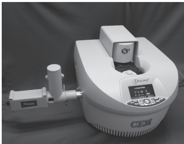
FIGURE 1.4 Example of a commercial microwave reactor with an integrated camera. Source: Acknowledgment is given to CEM Corporation for the generous loan of the microwave reactor for the construction of this text.
