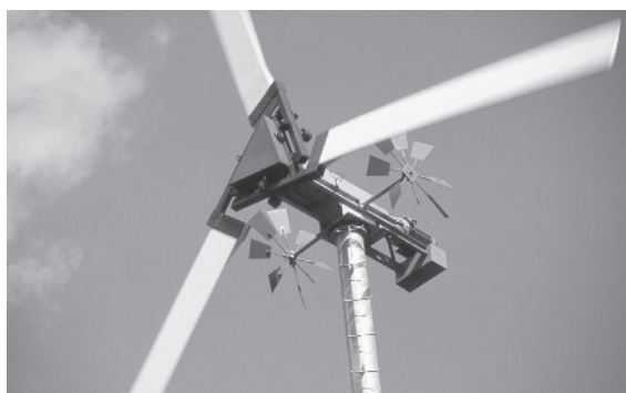
Figure 1.38 The early passively controlled wind turbine by Lagerwey van de Loenhorst with variable speed. Diameter: 10 m [8]
