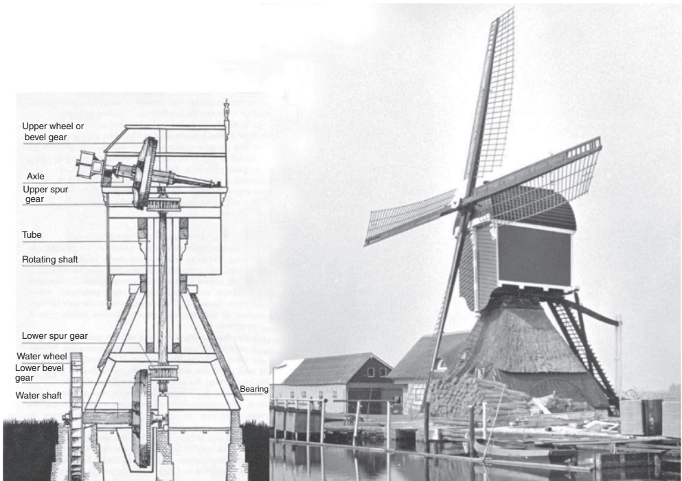
Figure 1.8 ‘Koker’ windmill from South Holland. Photo (right) from [8]
