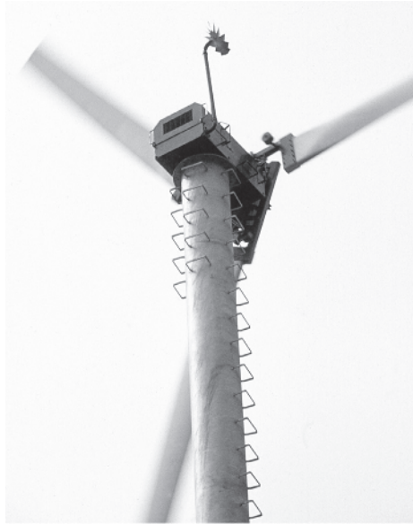
Figure 1.10 Wind direction follower with sensor on an early Lagerwey wind turbine [8]
