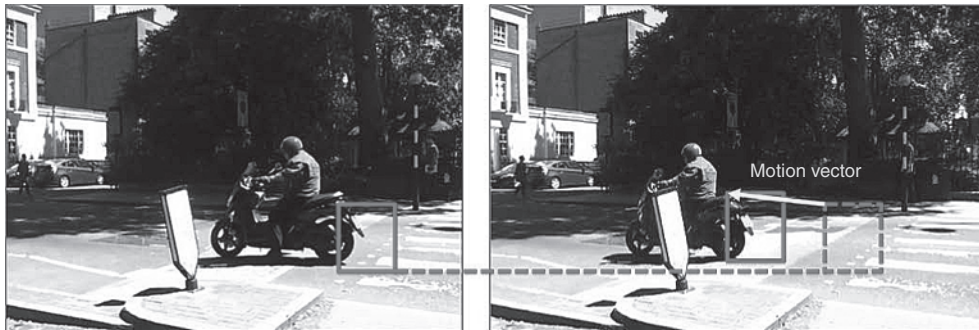
Figure 1.2 Motion estimation predicts the contents of each macroblock base due the motion relative to the reference frame. The reference frame is searched to find the 16 \times 16 block that matches the macroblock
