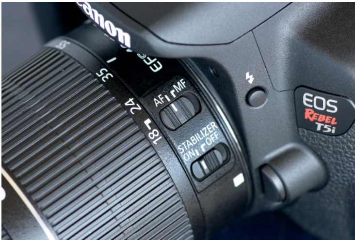
1.10 The Canon T5i/700D 18-55mm kit lens has Image Stabilization and focus switches on the left.
