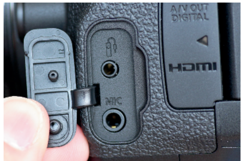
1.9 The connection terminals are located under the two covers on the left side of your camera.
