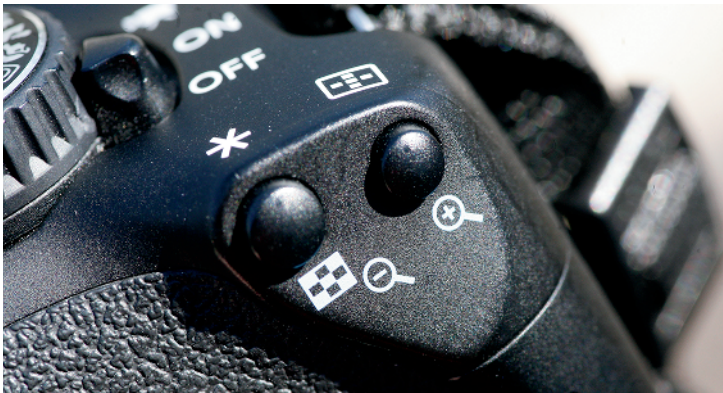
1.6 The Reduce/Exposure Lock/Flash Exposure Lock/Index and Magnify/Autofocus point select buttons are located on the back of your camera on the upper-right side.
