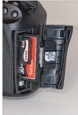
Figure 1-13: Inserting a memory card.
