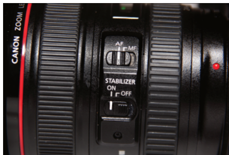
Figure 1-9: Slide this switch to enable image stabilization.
