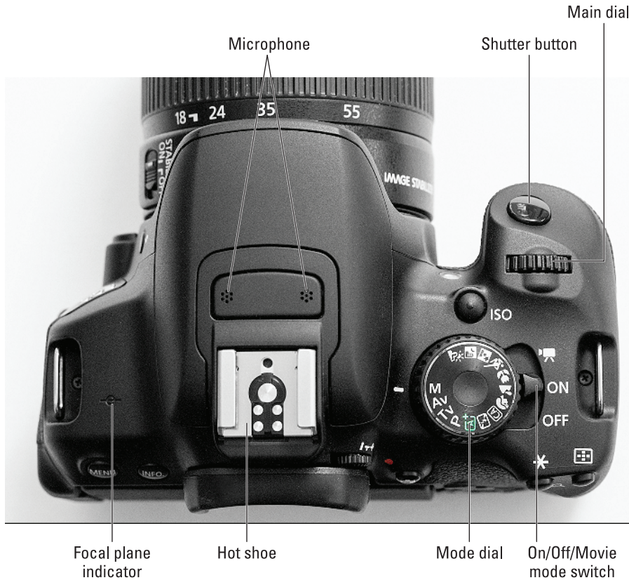
Figure 1-12: Here's a guide to controls found on top of the camera.
