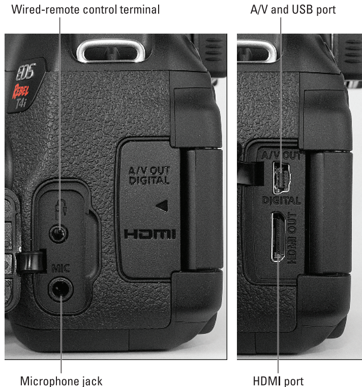
Figure 1-15: These two rubber covers conceal terminals for connecting the camera to other devices.
