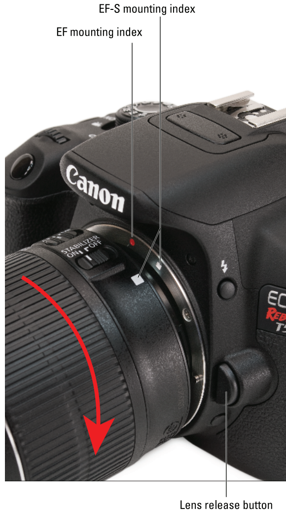
Figure 1-1: Place the lens in the lens mount with the mounting indexes aligned.
