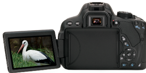
Figure 1-5: You also can unlock the monitor from the body and then rotate the screen to get the best view of things.
