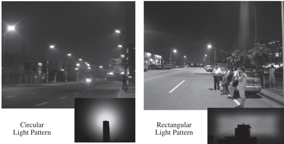
Figure 1.5 Illumination performances for LED road lighting with a (left) circular light pattern and (right) rectangular light pattern.
