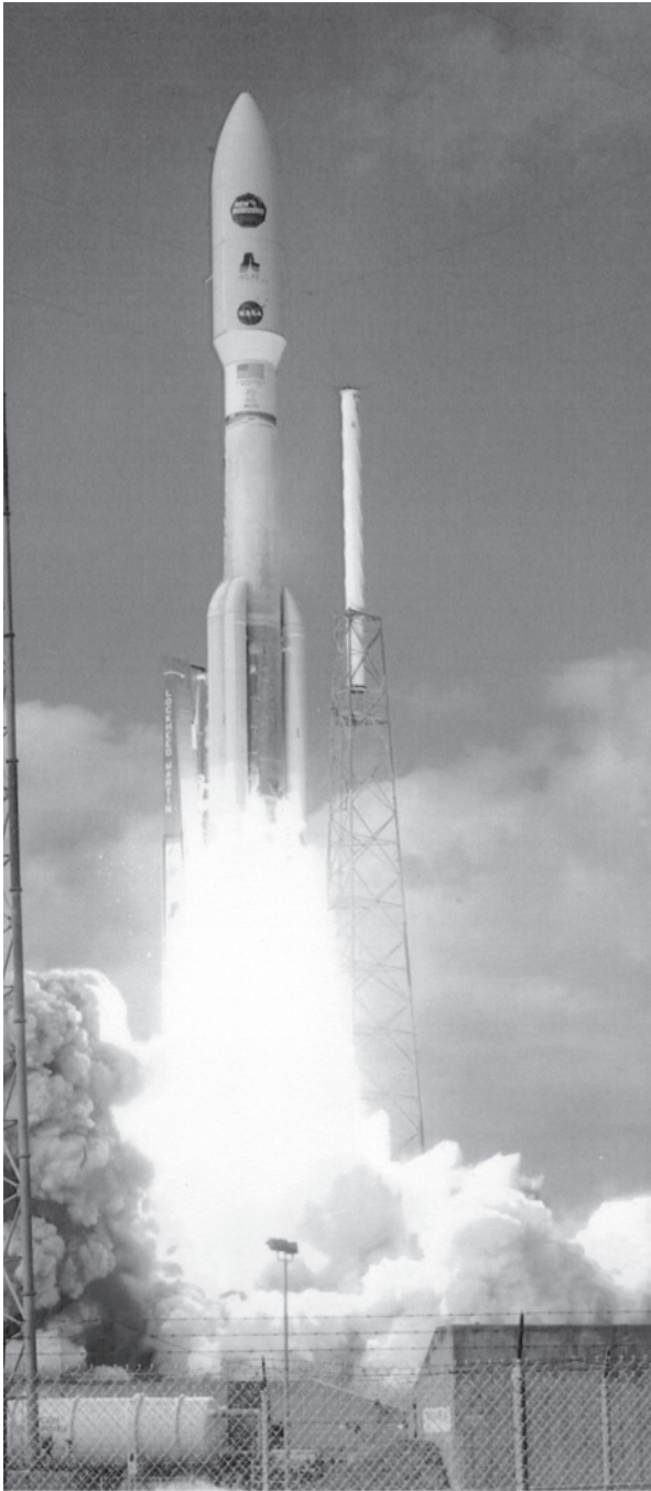
FIGURE 1–13. Atlas V space launch vehicle with three (or five) strap-on stages using Aerojet solid rocket motors and a central Energomash (Russia) RD-180 liquid propellant booster rocket engine running on LOX/kerosene. See Table 1–3 for key parameters. Courtesy United Launch Alliance.
