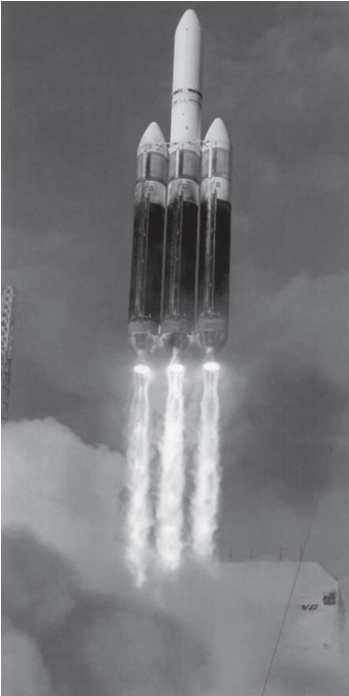
FIGURE 1–12. Delta IV HEAVY lift space launch vehicle. The center liquid propellant booster stage has a Pratt & Whitney Rocketdyne RS-68A rocket engine (LOX/LH 2 ). The two strap-on stages each use the same engine. See Figs. 6–9a and 6–9b. Courtesy Aerojet-Rocketdyne.
