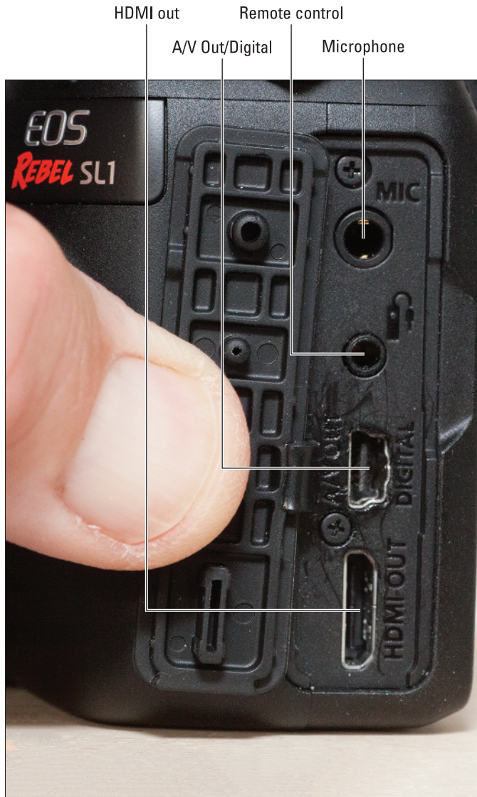
Figure 1-7: Ports just looking to be plugged.
