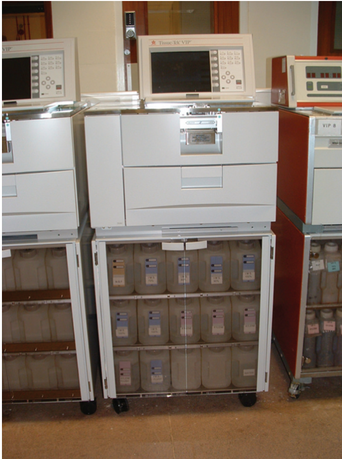
Figure 1.8 Machine for tissue dehydration, clearing and impregnation with paraffin wax.
