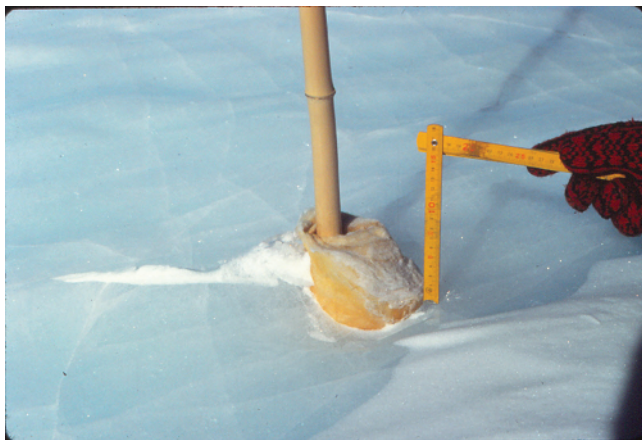
Figure 1.9. Measuring the 5-cm ablation of ice at a flagpole of the geodetic net.
