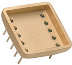
(a) Kovar package with metal-in-glass feed-throughs. The Kovar is gold-plated; lid usually resistance-welded to wall.
