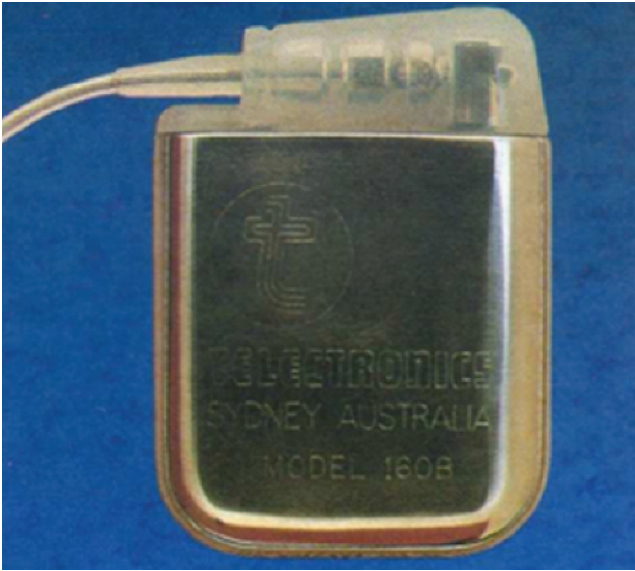
Figure 1.2 The first modern pacemaker was made by Teletronics in 1971. The engineer David Cowdrey, who had been charged with developing a hermetic enclosure, selected Ti because of its light weight, strength, corrosion resistance and weldability. He used deep-drawn Ti half-cases that were welded together using TIG welding to keep the inside cool. He also developed ceramic/Ti alloy feed-throughs for the package. Interestingly, the technology was never patented because the company's patent attorney advised them that it "was obvious"! This picture shows a Teletronics 'Slimline' device from 1977.
