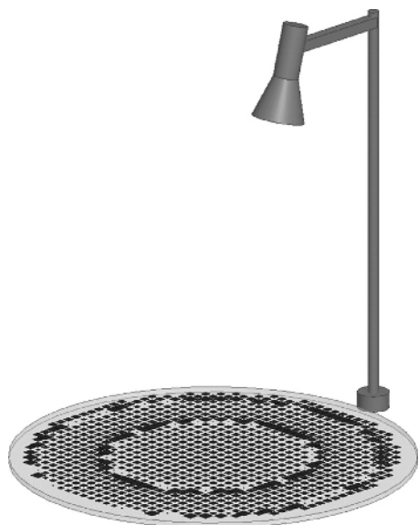
Figure 1.1 The geometry of an offset-fed reflectarray antenna.
