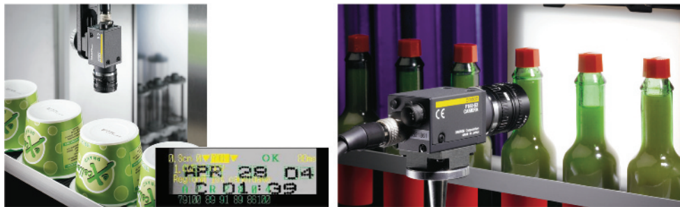
Figure 1.3 Checking print quality of best-before dates (right), and monitoring level to which bottles are filled (right). Reproduced by permission of Omron Electronics LLC
