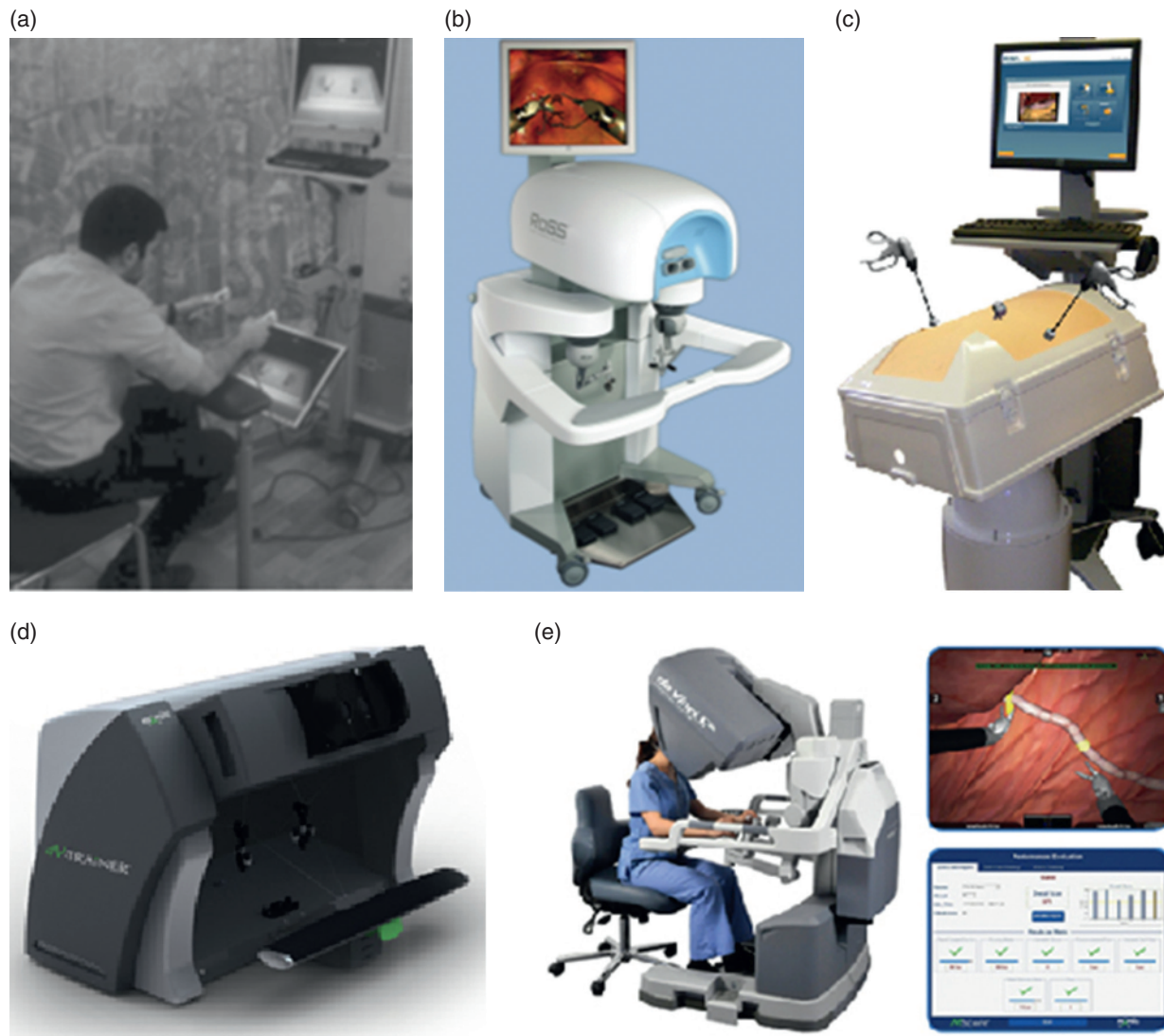
Figure 1.3.1 Virtual reality robotic simulators. (a) SEP, (b) RoSS, (c) ProMIS, (d) MdVT, (e) dVSS.
