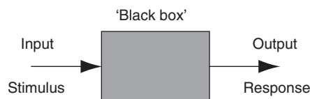
Figure 1.2 A black-box element with an input–output relationship.
