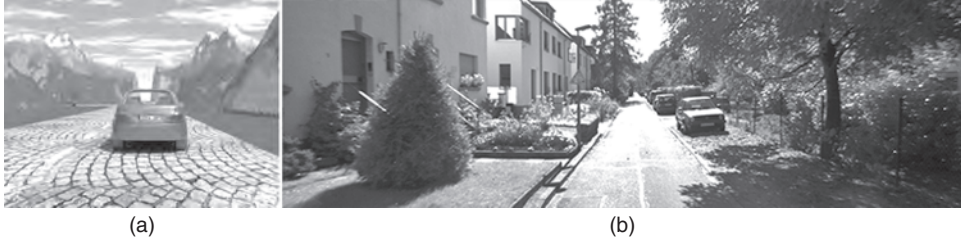
Figure 1.4 Examples of benchmark data available for a comparative analysis of computer vision algorithms for motion and distance calculations. (a) Image from a synthetic sequence provided on EISATS with accurate ground truth. (b) Image of a real-world sequence provided on KITTI with approximate ground truth
