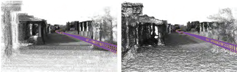
Figure 1.9 (a) Reconstructed cloud of points. (b) Reconstructed surface based on a single run of the ego-vehicle. Courtesy of Yi Zeng
