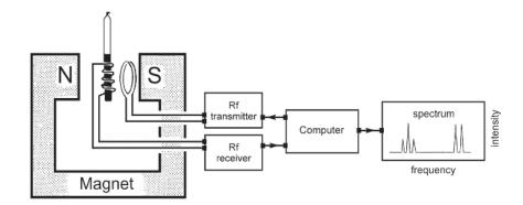
Magnets for NMR spectroscopy may be either permanent magnets or electromagnets. Most modern magnets are electromagnets based on superconducting solenoids, cooled to liquid helium temperature.
