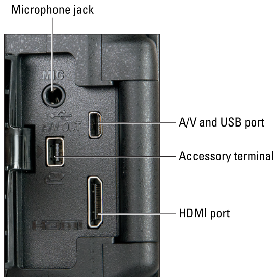
Figure 1-8: Open the cover on the side of the camera to reveal these connections.
