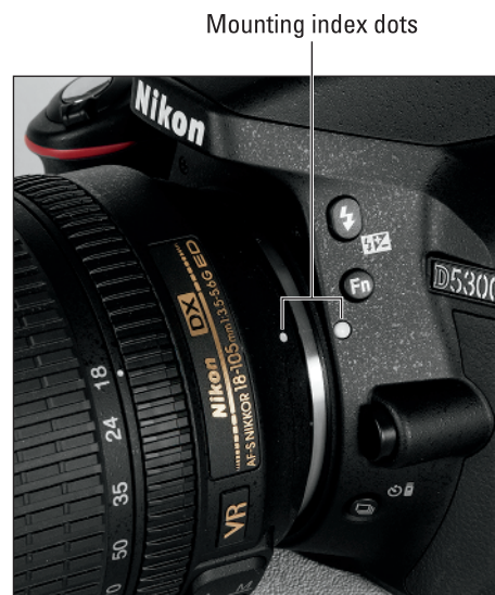
Figure 1-1: Align the white dot on the lens with the one on the camera body.
