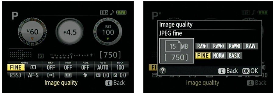
Figure 1-14: Press the i button to activate the control strip (left); highlight the option you want to adjust and press OK to display the available settings (right).
