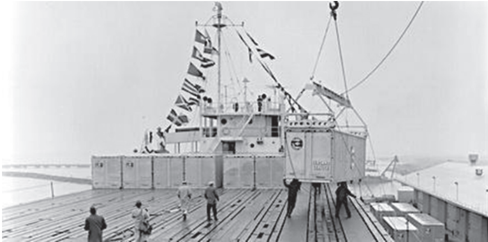
Figure 1.2 The Ideal-X loading the first ever containers (“the box”) at the Newark, NJ, port for their maiden voyage to Houston, Texas, April 26, 1956. Source: The Port Authority of New York and New Jersey.
