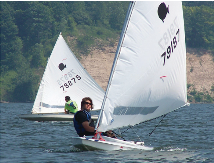
FIGURE 1.1 A Dhow sailing vessel with Lateen rigged sails (a) and one of the most popular recreational sailboats, the Sunfish (b), which use the same ancient sail design. This was the first sail design that allowed sailboats to tack (go back and forth at an angle) allowing travel upwind. Modern wind turbines are driven by similar crosswind (lift) forces. See more about lift forces in Figure 4.5 (Photo Credit—upper photo: Xavier Romero-Frias, http://en.wikipedia.org/wiki/File:Sd2-baggala.JPG ; lower photo: Dierde Santos, http://en.wikipedia.org/wiki/File:SunfishRacing.jpg ).
