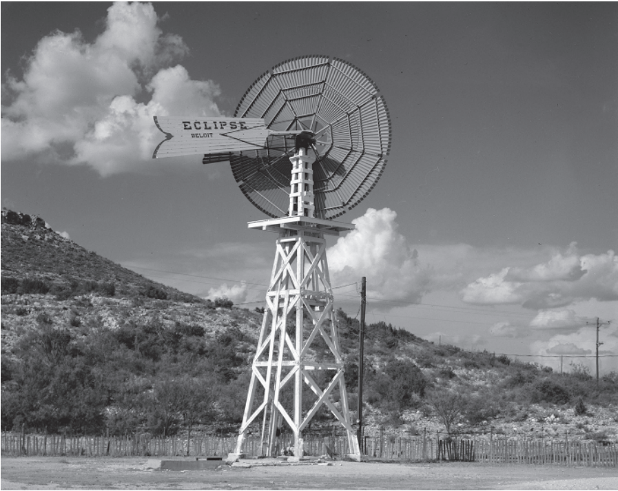
FIGURE 1.6 Eclipse wind pumper (Courtesy of I.G. Holmes, U.S. National Park Service).
