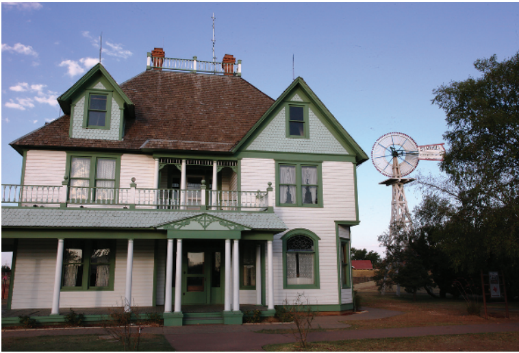
FIGURE 1.8 Windmill used for water pumping to a nineteenth century ranch home. Texas Tech University, National Ranching Heritage Center, Lubbock, TX (Charles Norland, Norland Photographic Art, St. Louis, MO. Picture taken at the National Ranching Heritage Center in Lubbock, TX).
