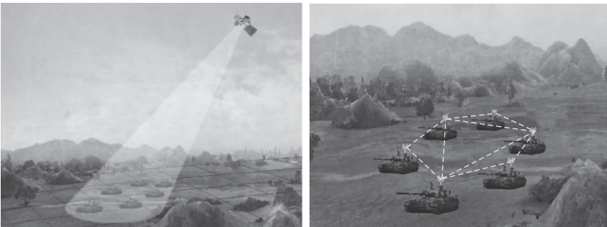
Figure 1.3 Centralized (left) and decentralized (right) formation control.
