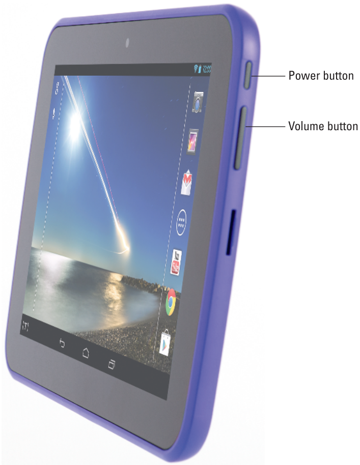
Figure 1-3: The only controls on the Hudl's case are the power and volume buttons.
