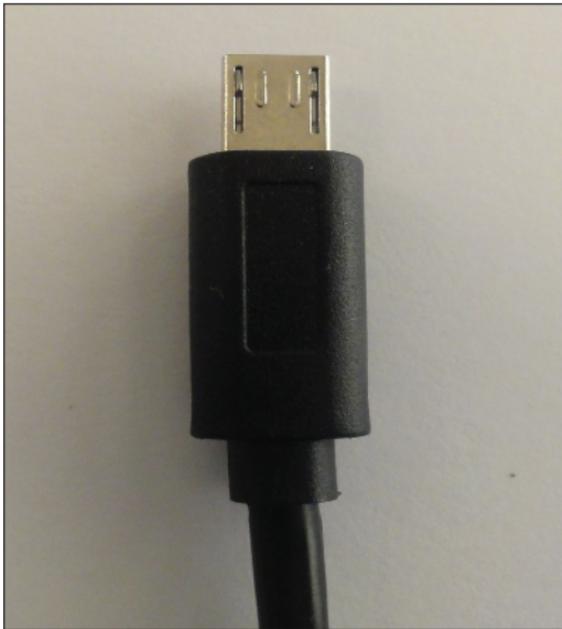
Figure 1-5: Make sure that you have the ridged side of the micro-USB connector uppermost when plugging it into the Hudl.
