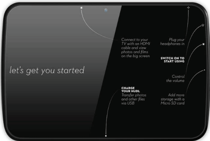
Figure 1-2: Get to know the buttons and ports on your Hudl before you begin.
