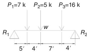
**FIGURE 1.23** Simple beam various loads resultant forces.
