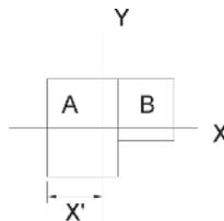
**FIGURE 1.6** Center of gravity determining  $X$ .
