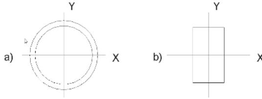
**FIGURE 1.3** Center of gravity of pipes and rectangles.
