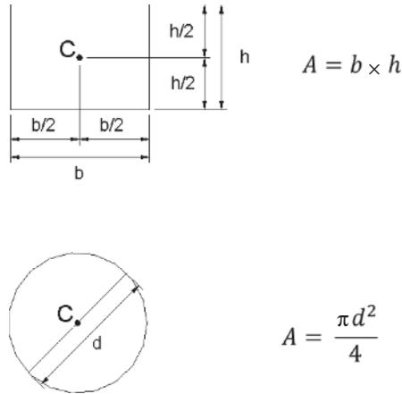
FIGURE 1.8 Centroids of area of common shapes.
