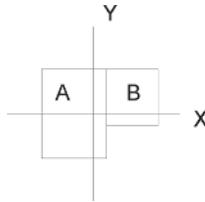
**FIGURE 1.4** Center of gravity of a composite shape.
