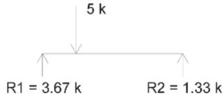
**FIGURE 1.21** Simple beam resultant force solution.
