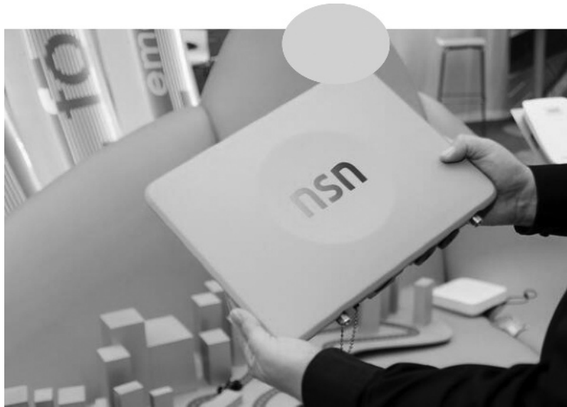
Figure 1.9 The LTE micro cell base station with 5 kg, 5 L and 5+5 W
