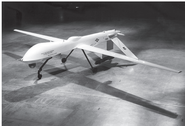
Figure 1.1 General Atomics RQ-1A Predator. (Photo: USAF Museum). (See insert for color representation of this figure.)
