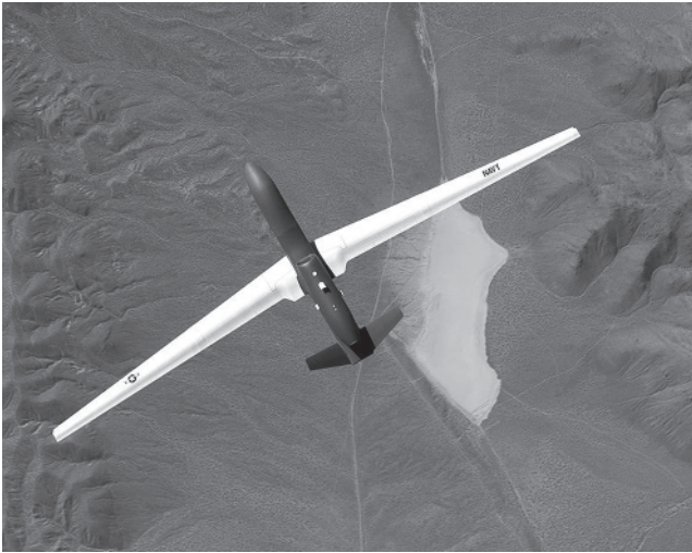
Figure 1.5 Sweptback tapered planform in a Northrop Grumman RQ-4 Global Hawk. Photo: Jim Gordon.
