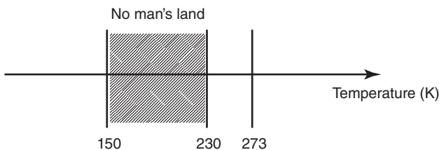
Figure 1.1 Schematic description of the so-called “No man’s land” of water between 150 and 230 K. In this region crystallisation of bulk water and aqueous solutions of higher water contents cannot be avoided. 273 K is the melting temperature of bulk water.
