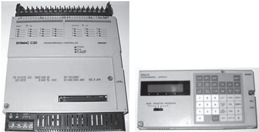
Figure 1.2 Omron Sysmac C20—Nonmodular PLC with digital I/O and programming terminal
