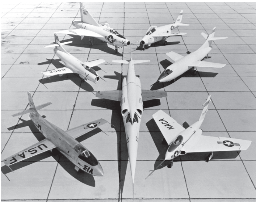
Figure 1.10 Early X-planes, including the Douglas X-3 Stiletto (center) and (clockwise, from lower left) Bell X-1A, Douglas D-558-1 Skystreak, Convair XF-92A, Bell X-5, Douglas D-558-2 Skyrocket, and the Northrop X-4 Bantam. Source: NASA.
