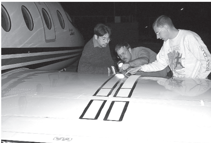
Figure 1.7 Inspection of pressure-sensitive paint on Purdue University’s Beechjet 400 following a flight test in 1999 (depicted left to right are Hirotaka Sakaue, Brian Stirn, and Jim Gregory). Source: Photo courtesy of Nate Lachendro.
