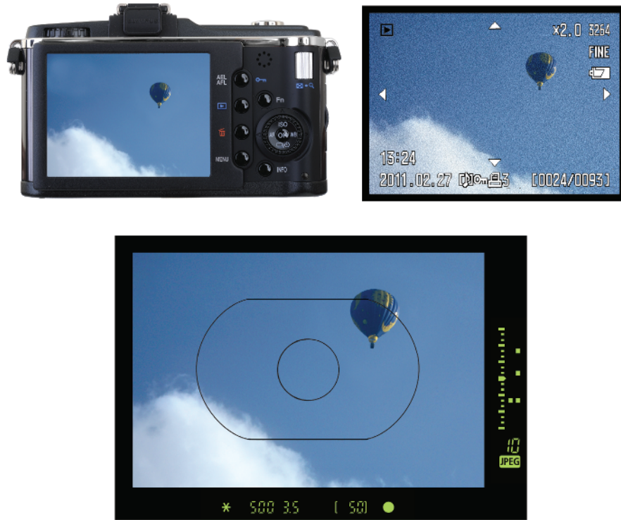
Figure 1-2: A back panel LCD viewfinder (upper-left) or an EVF LCD (upper-right) is no match for a dSLR's optical system (bottom).
