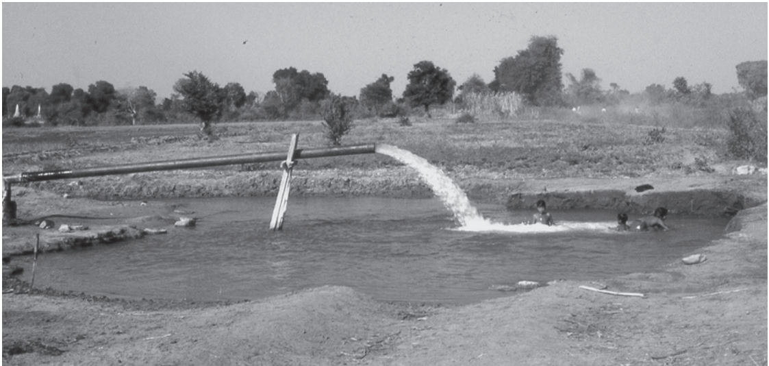
Figure 1.7 Flowing artesian well, northern Myanmar. The well was drilled into a strongly confined sandstone aquifer. Children are enjoying the 'swimming pool' created by the discharge until such time as the well is capped. Photo by Bruce Misstear
