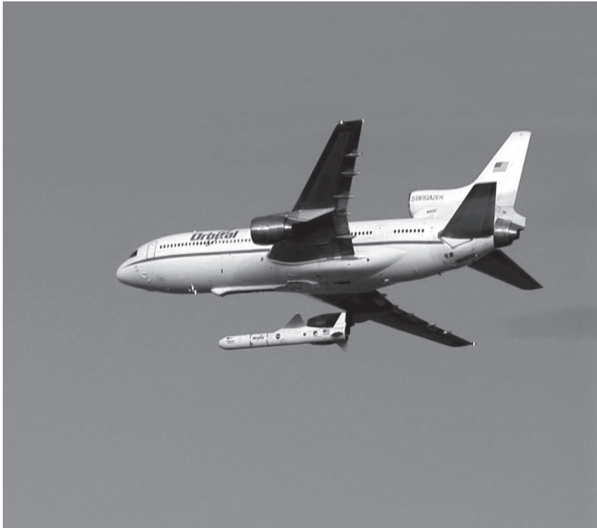
Figure 1.80 Orbital Sciences ASB-11 Pegasus launch vehicle dropped from Lockheed L-1011 carrier aircraft. (Source: NASA.)
