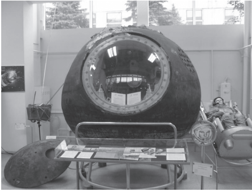
Figure 1.65 Russian Vostok 1 , the first manned spacecraft on display at the RKK Energiya Museum, Moscow, Russia. The capsule hatch, on the ground at left, is replaced by a clear window. The ejection seat is on the right. (Source: © D.R. Siefkin, “Gagarin Capsule” https://en.wikipedia.org/wiki/File:Gagarin_Capsule.jpg , CC-BY-SA-3.0. License at https://creativecommons.org/licenses/by-sa/3.0/legalcode .)
