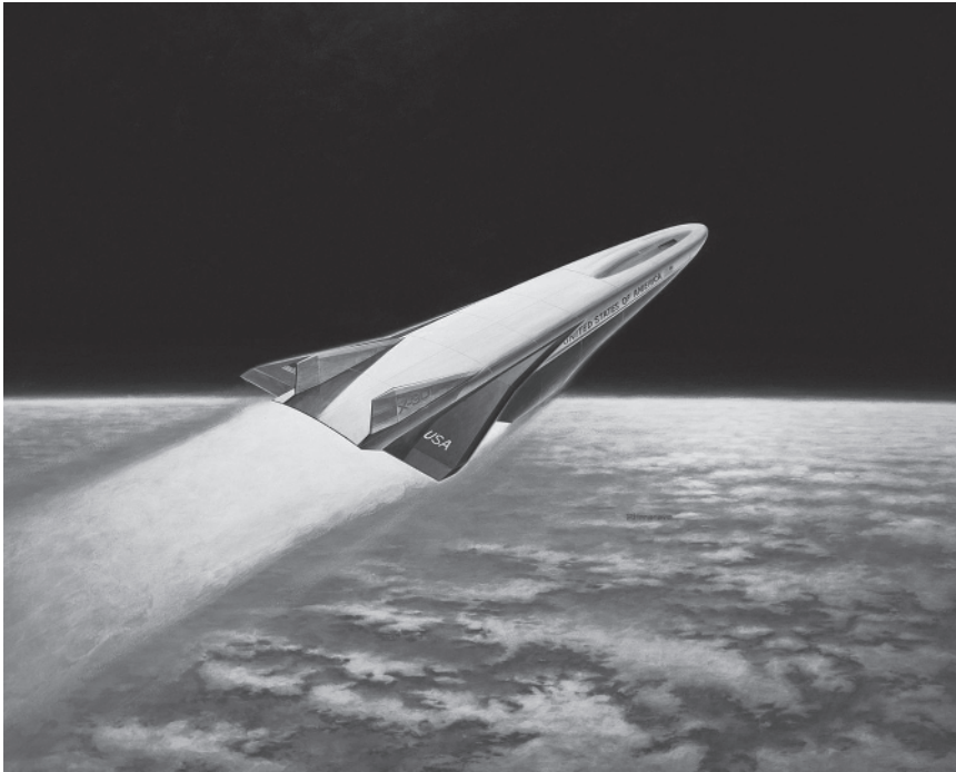
Figure 1.83 The X-30 National Aerospace Plane single-stage-to-orbit concept, 1990. (Source: NASA.)
