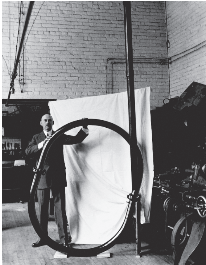
Figure 1.73 Robert Goddard with vacuum tube device, which he used to prove that a rocket could produce thrust in the vacuum of space, June 1916. (Source: NASA.)
