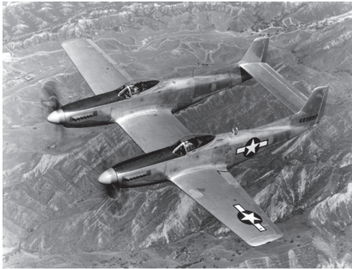
Figure 1.15 North American F-82 Twin Mustang twin fuselage airplane. Note that there is a pilot in each fuselage cockpit. (Source: US Air Force .)
