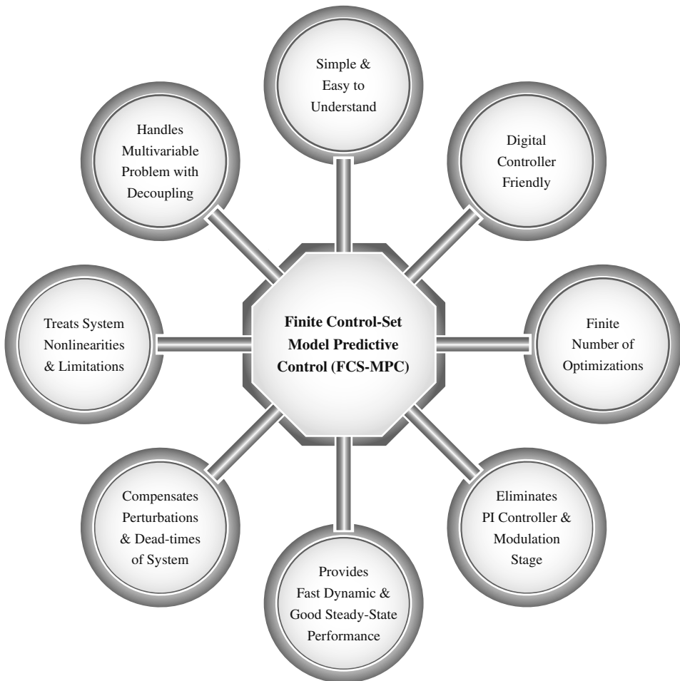
Figure 1.29 Main features of finite control-set model predictive control.
