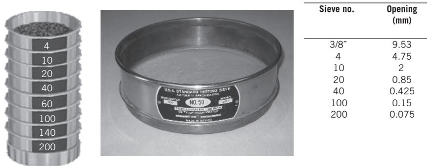
Figure 1.6 Stack of US sieves.
