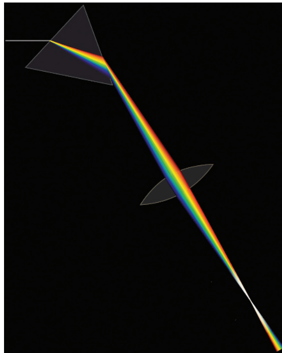
Figure 1.1 Splitting and recombining white light with a prism and a lens respectively.
