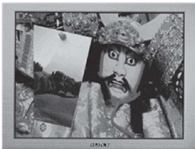
Figure 1.4 A 13” active-matrix full-color OLED display developed by Sony in 2001 [9]. (provided by Sony Corporation)
