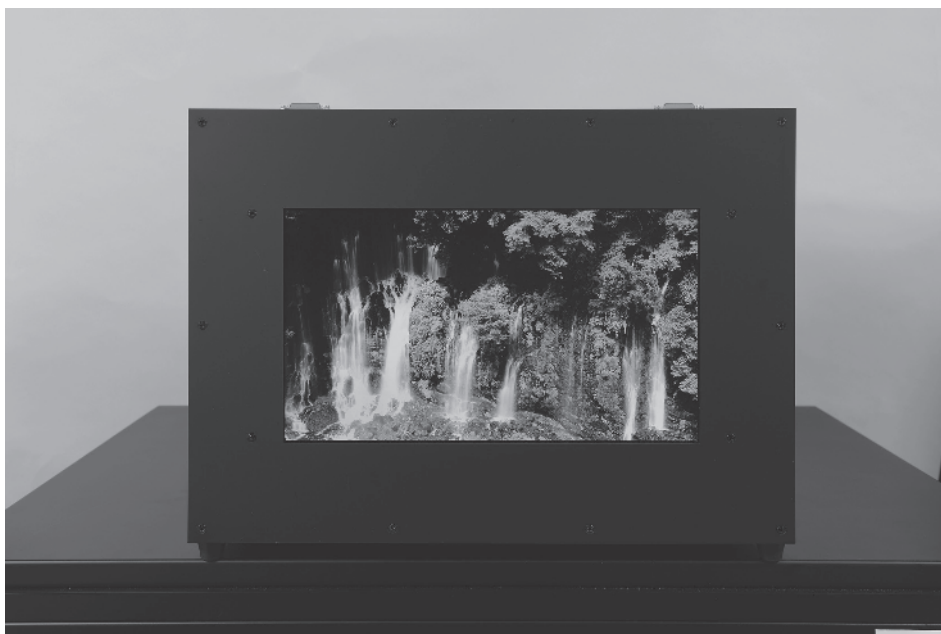
Figure 1.7 Prototype of 13.3" AM-OLED display with 8K format (Semiconductor Energy Laboratory & Sharp) [25]. (provided by Semiconductor Energy Laboratory)
