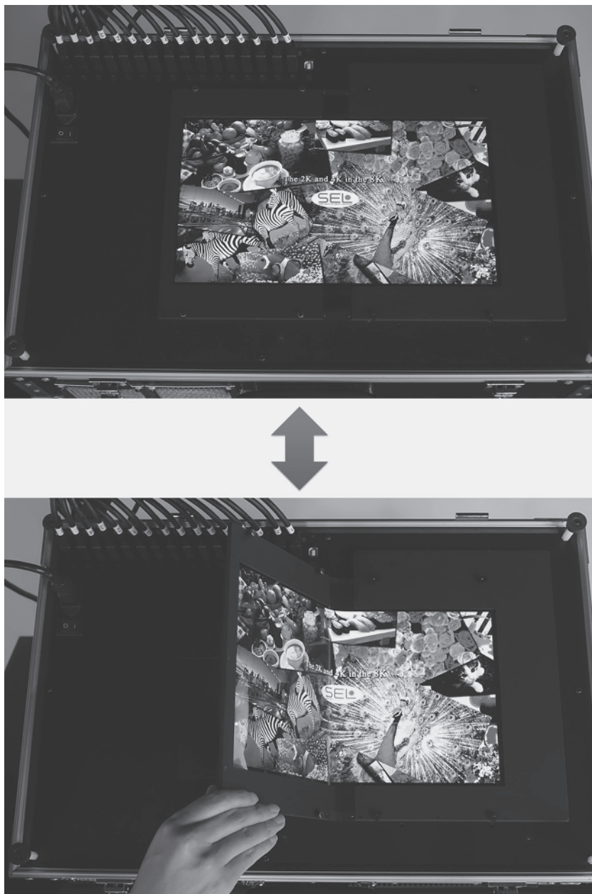
Figure 1.10 Prototype of 13.3" foldable AM-OLED display with 8 K format (Semiconductor Energy Laboratory) [29]. (provided by Semiconductor Energy Laboratory) Display size: 13.3" (165 mm×294 mm) Number of pixels: 4320×7680 (4k8k) Resolution: 664 ppi Color: full color Device structure: white tandem OLED (top emission)+color filter Driving: active-matrix with CAAC-IGZO TFT
