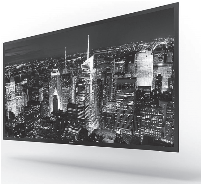
Figure 1.6 A 56" active-matrix full-color OLED display with 2K4K format developed by Sony in 2013. (provided by Sony Corporation)
