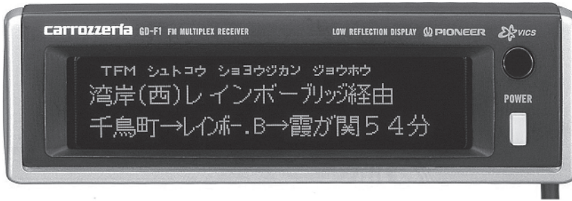
Figure 1.2 The world's first OLED product (passive-matrix OLED display for car audio) commercialized by Pioneer in 1997 [6]. (provided by Pioneer Corporation)
