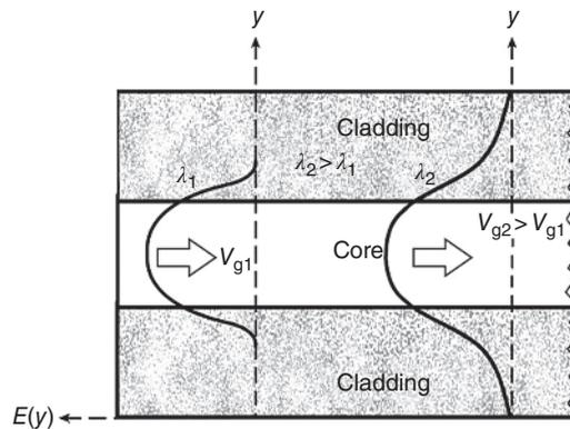
**Figure 1.9** Electric field of a fundamental mode through a slab waveguide at different wavelengths ( $\lambda_1$  and  $\lambda_2$ ) where ( $\lambda_1 < \lambda_2$ )
