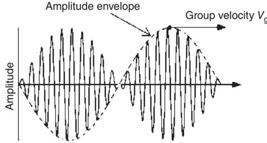
**Figure 1.7** The superposition of two waves of different frequencies
