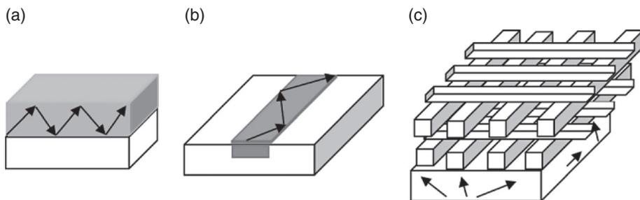
**Figure 1.3** Common waveguide geometries based on light confinement: (a) planar waveguide, (b) rectangular channel waveguide, and (c) photonic crystals
