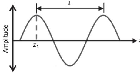
**Figure 1.5** A traveling wave along the  $z$ -axis
