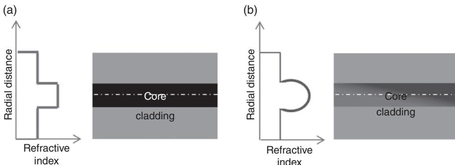
**Figure 1.4** Classification of optical waveguide based on the refractive index distributions: (a) step-index optical fiber and (b) graded-index optical fiber
