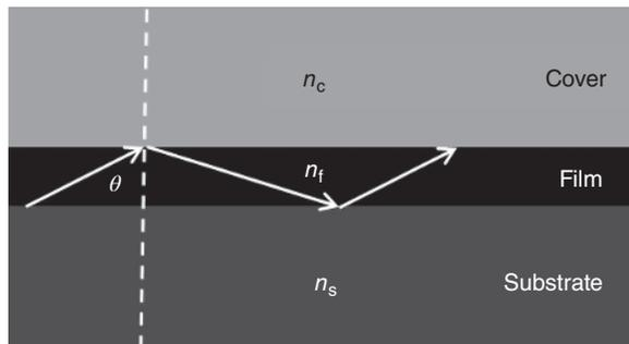
**Figure 1.8** Zigzag trajectory of a confinement ray inside the film of a planar waveguide
