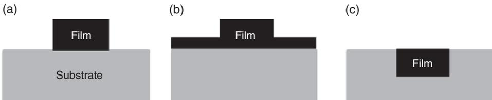
**Figure 1.2** Common channel waveguides: (a) strip, (b) rip, and (c) buried
