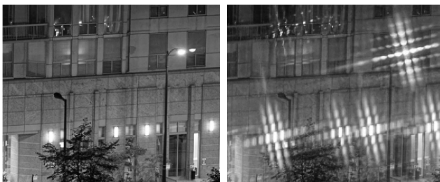
Figure 1.10 View of streetlamps from a hotel room in Chicago in 2010. The image on the right side is the exact same view as the one on the left; only it was taken through the curtain fabric. All strong and point-like light sources show significant diffraction.
