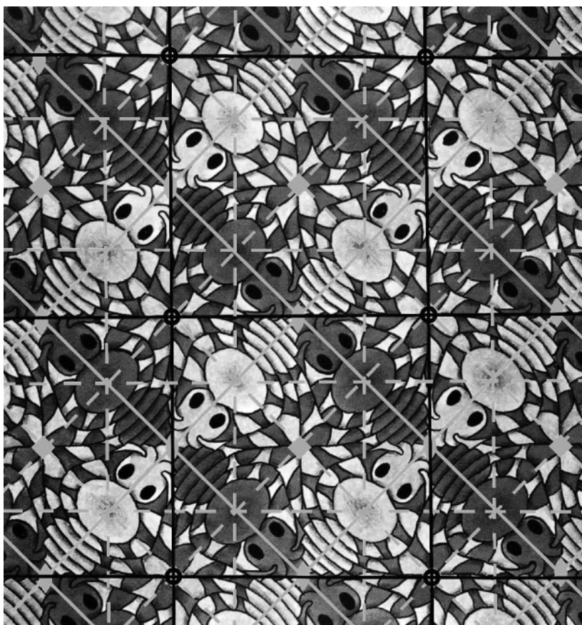
Figure 1.5 Wallpaper design by M. C. Escher. Assume the grey and white spiders are equivalent and a symmetry operation transforming a grey spider into a white one or vice versa is considered valid. Lattice points are indicated by black circles; the lattice is drawn as black lines. Symmetry elements are drawn in white (fourfold axes, twofold axes, mirrors, and glides). The lattice type is square and the plane group is p4gm . Each unit cell contains 4 spiders, the asymmetric unit \frac{1}{2} spider. Source: M.C. Escher's "Symmetry Drawing E86" © 2018 The M.C. Escher Company-The Netherlands. All rights reserved. www.mcescher.com .
