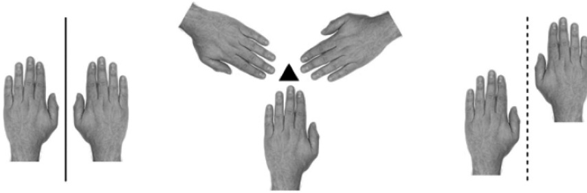
Figure 1.3 Symmetry operations of mirror, threefold rotation, and glide are depicted on a photograph of a hand. The symbol for a mirror is a solid line, for a threefold rotation a triangle ( \blacktriangle ), and for a glide a dashed line.
