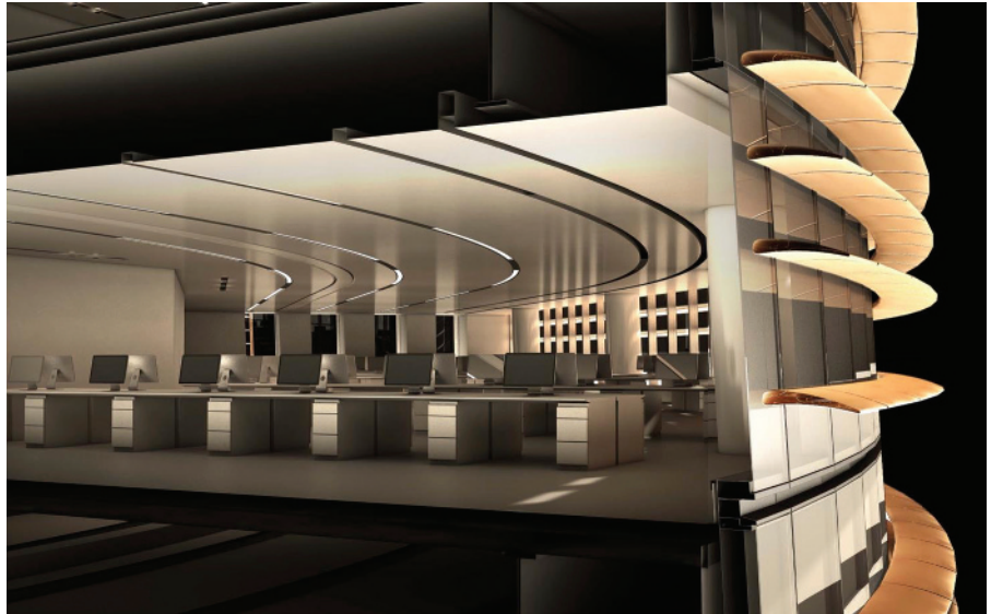
Figure 1.12 The actual designed fixed external fin system wraps around each floor of the building, terminating at the east and west notches. (Source: SOM)
