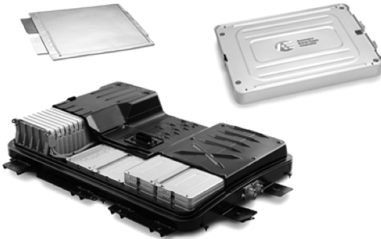
FIGURE 1.23 Nissan Leaf battery cell, module, and pack. Upper left: a laminated battery cell; upper right: a battery module set of four laminated battery cells; bottom: a battery pack made up of 48 modules. (Reproduced from Ref. [55] with permission from IEEE.)
