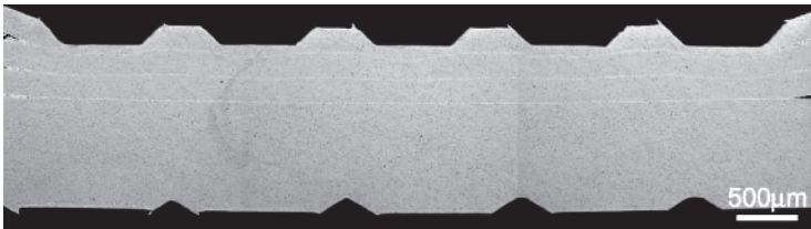
(b) Optical micrograph of a four-layer copper USMW (Reproduced from Ref. [26] with permission from Elsevier.)
