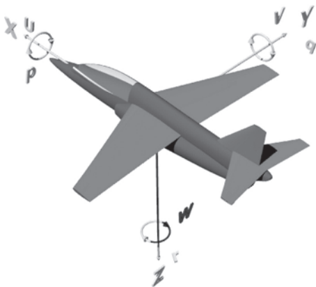
■ TABLE 1.6 Summary of the components of the six degrees of freedom in the body-fixed coordinate system, F_B
