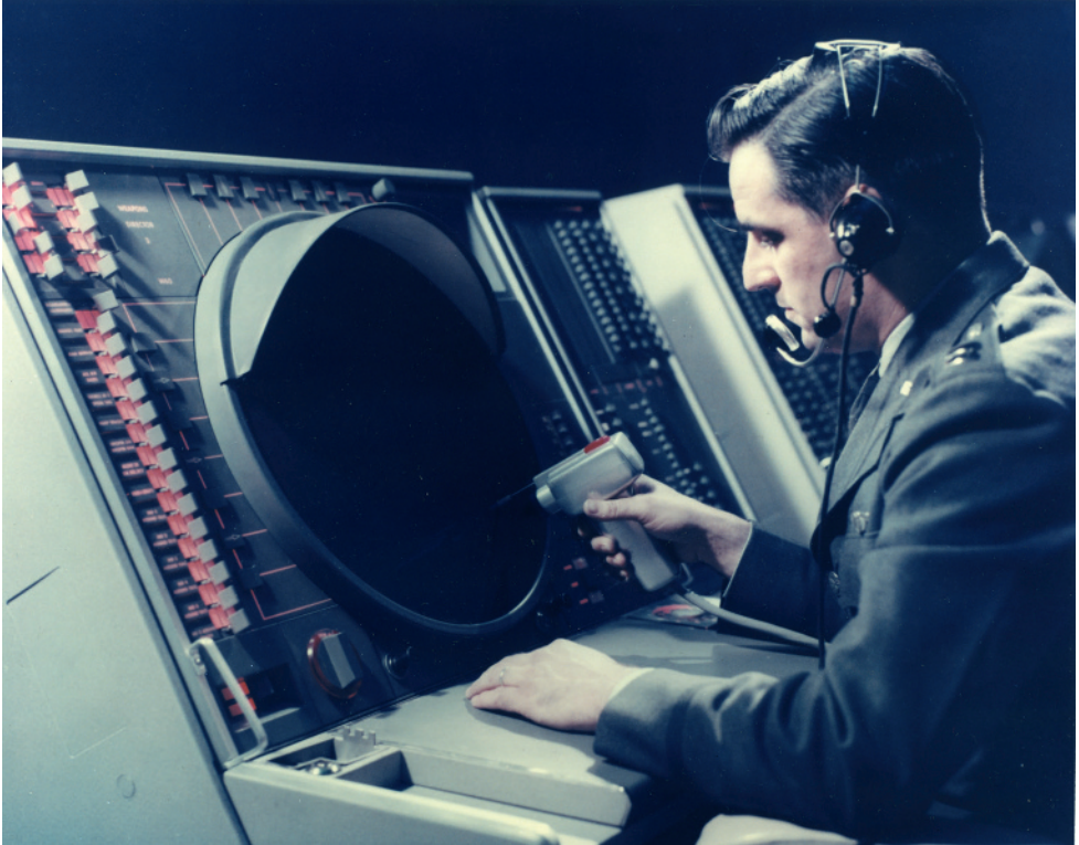
View of a control room of the SAGE system, 1959 On the screens of the SAGE system, one of the very first large-scale computer networks, operators could monitor events and situations related to the defence of North American airspace.
