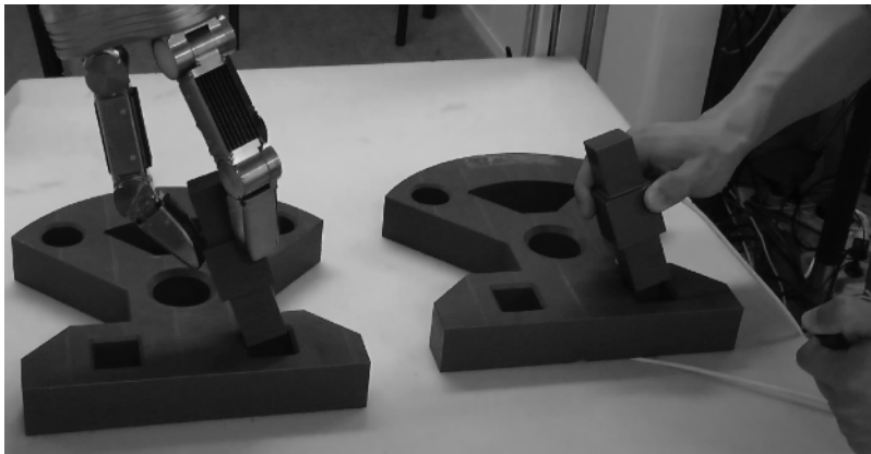
Figure 1.5 The PbD setup for teaching peg-in-hole assembly tasks includes a teleoperated robot gripper and the objects manipulated by a human expert. Tracking is done using magnetic sensors. (Yang et al. (2014). Reproduced with permission of IEEE.)
