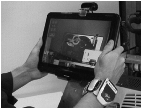
Figure 1.8 Mobile AR component including a haptic bracelet. (Webel et al. (2013). Reproduced with permission of Elsevier.)
