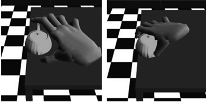
Figure 1.16 Robot grasp planning application. (Aleotti and Caselli (2010). Reproduced with permission of Elsevier.)
