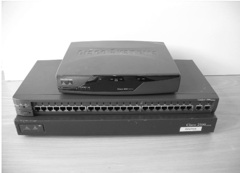
FIGURE 1.1 Cisco routers and switches
